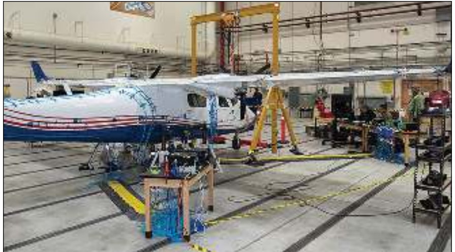
Overview of GVT setup on the X-57 Maxwell Mod II Configuration. (Image: Courtesy of NASA)
