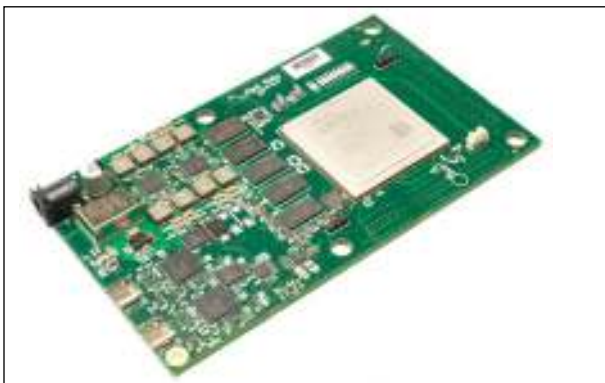
The XEM8350 is based on the Xilinx Kintex UltraScale FPGA and includes dual SuperSpeed USB 3.0 interfaces, on-board DDR4 memory, and over 330 user I/O.
