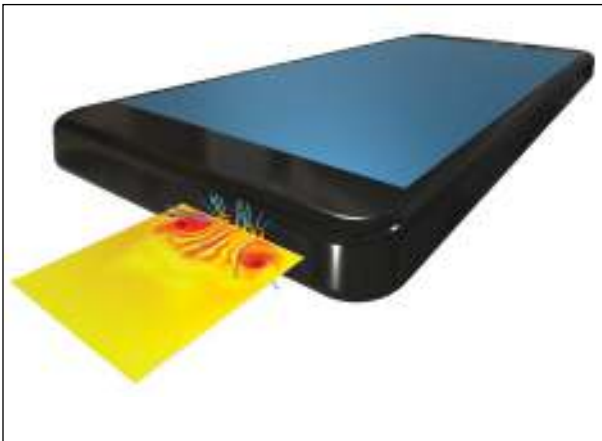
Multiphysics simulation of microspeaker acoustics taking into consideration the nonlinear thermoviscous acoustics effect
